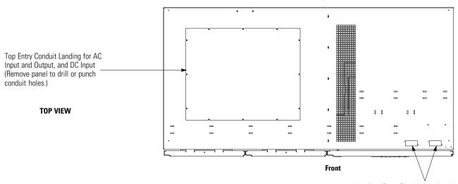
Interface Entry Conduit Landings for TB1 through TB3 Wiring and X-Slot Connections (Remove panels to drill or punch conduit holes.)
